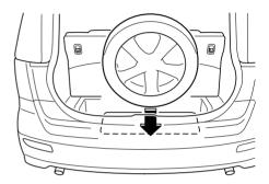
10. Thread the belt through the wheel as shown in the figure, then attach the belt clips to the cargo securing loops on the back of the third-row seat.
